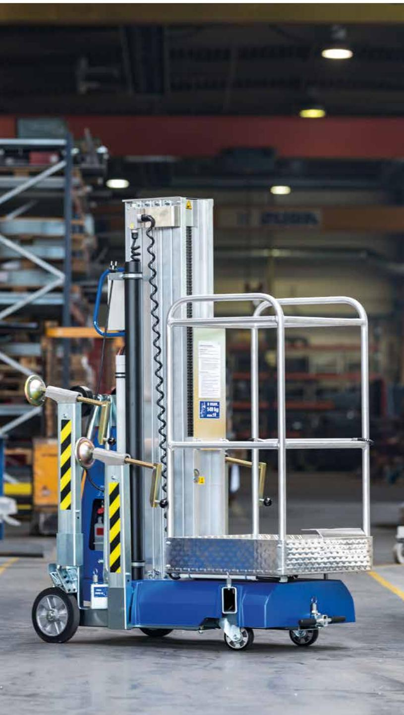
For maintenance and repair work, the ALP-Personnel-Lifts are practically indispensable, in particular in enclosed rooms with high ceilings. Whether installation, repair, maintenance or cleaning, with the Böcker ALP-Lifts you will reach the optimal operating height at all times. On-site, the equipment is immediately operational and thanks to user-friendly operation, they offer maximum efficiency and high operating speeds.
