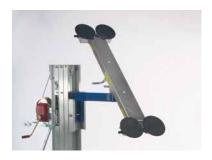
Manual gas suction unit for overhead glazing
