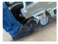
Fixing of the locking brake at the swivel castor
