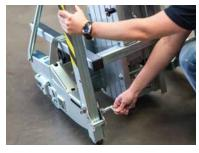
Opening and fixing of front sections by means of spring locking bar
