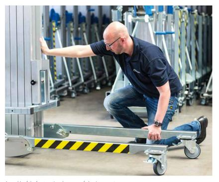
Assembly of the front sections by means of plug-in connectors  $% \left( 1\right) =\left( 1\right) \left( 1\right$
