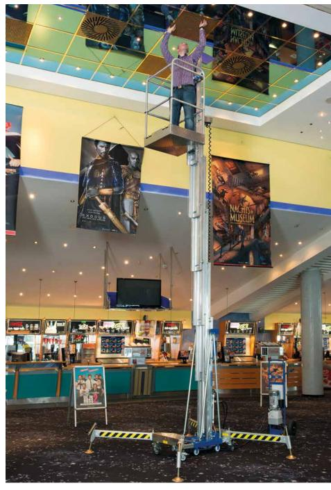
For the use on level surfaces, the ALP-Personnel-Lift PHC 1000 EU can be extended with an adapter unit with outriggers.
